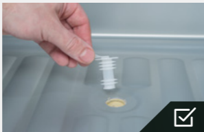
Drainage hole with hose connector (bottom)
